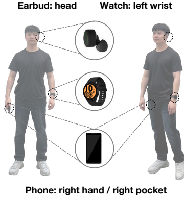
Figure 6: ULTRAPOSER system setup. ULTRAPOSER collects data from users wearing a smartphone, smartwatch, and earbud. The smartphone is either held in the hand or placed near the trouser pocket during data collection.
